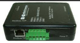
Figure 4. MES1B Serial Connector
